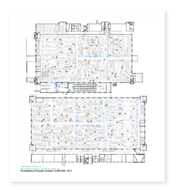
Identify choke points and man / machine collision risk areas in a factory or distribution center setting
